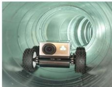
Chassis with 2 cameras and Strong LED lamp. Control box with joystick and light adjustment and 30 meters cable.
