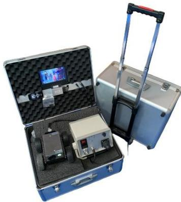
The robot is easily operated from the control box where a joystick allows you to take the robot in whatever direction you want. The intensity of the strong lamp on the robot is adjustable from the control box allowing you to adjust the light to the conditions as you go on.
