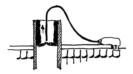
When the chimneys on the inside are covered in soot, you can use a rotating brush system with chains.
