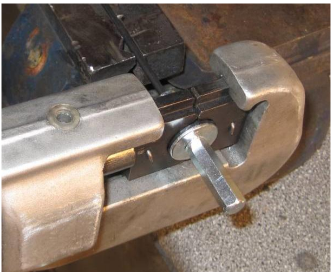
Press the coupling for shaft on the innercore using the prestool
