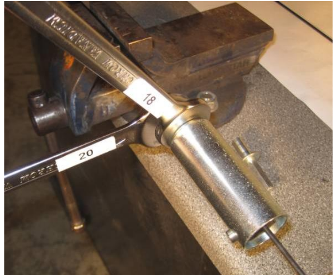
Assemble the Screw-joint and the coupling for hose using a 20 and 18 wrench.
