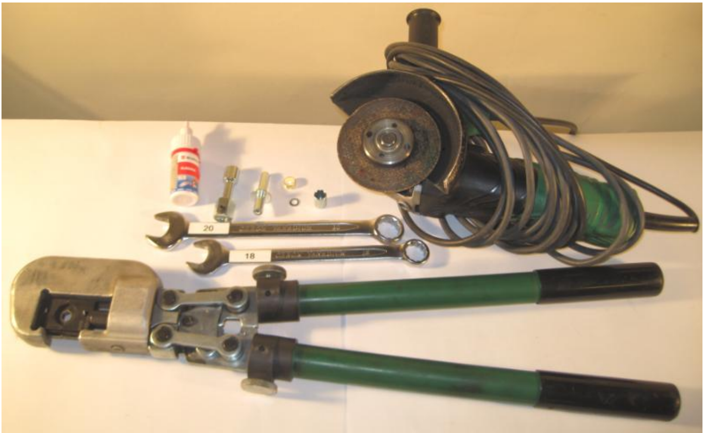
Tools which is needed for repairing the shaft
