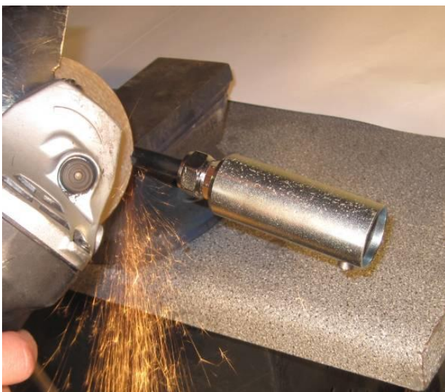
Cut the shaft at the break near the motor end
