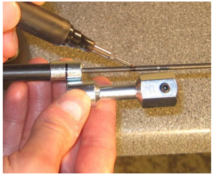
Use the connector for the brush to mark the length – as shown on the picture.
