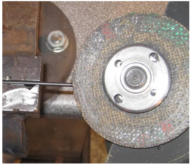
Grind the innercore to make a "bottleneck"
