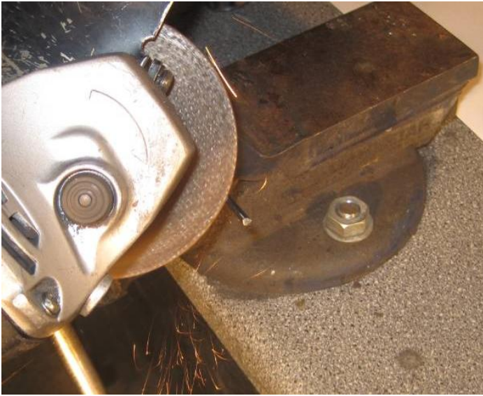
Grind the innercore to make the innercore round in the end.
