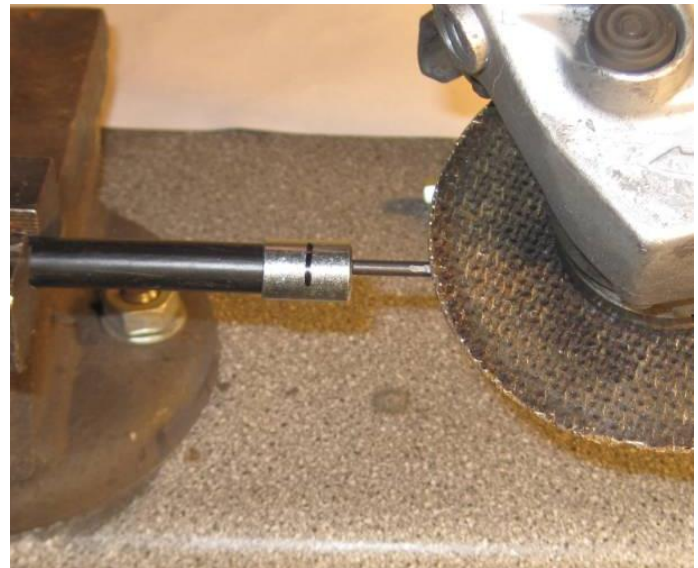
Grind the innercore making a bottleneck
