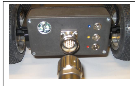
2. Connect the robot cable
