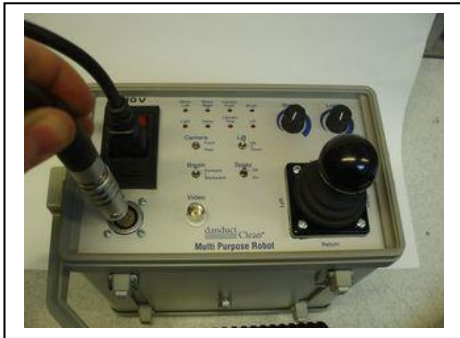
3. Connect the robot cable
