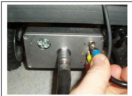
3. Fasten the motor plug
