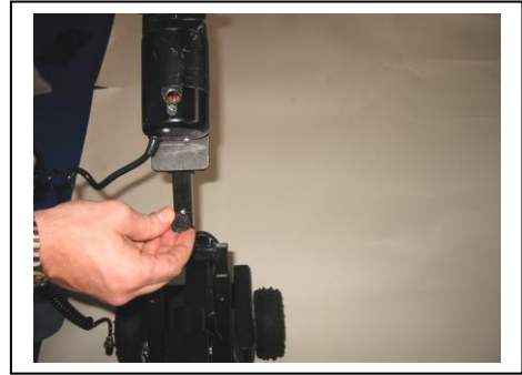
8. Mount motor and fasten screw
