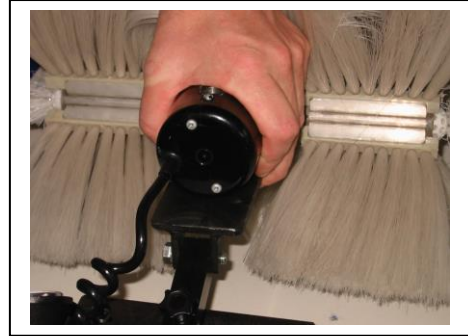
8. Adjust motor angle by hand
