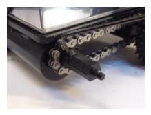
Use an alum wrench to tighten the chain wheel hub.
