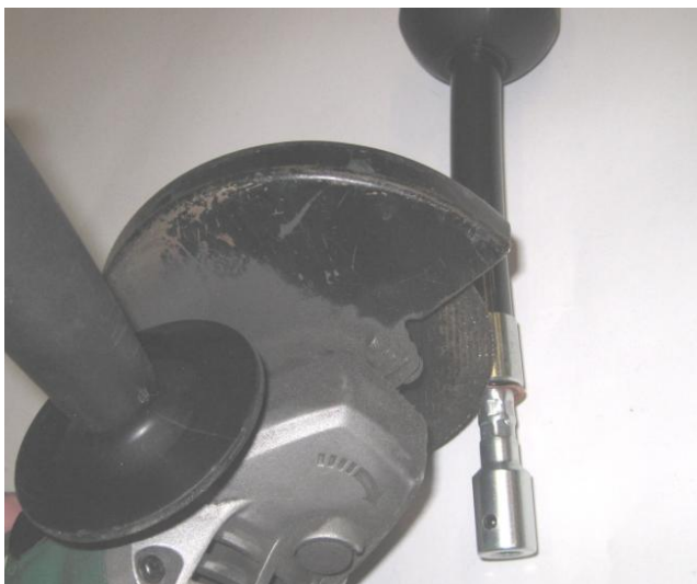
Cut the broken shaft at the Brush end.
