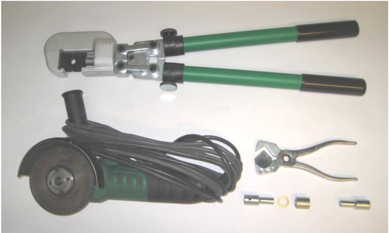
Tools needed in order to repair the shaft in the Brush-end
