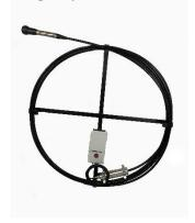
The signal from the miniature camera in the camera head is transmitted through a wire inside the hose to the power supply. From the power supply the signal is transmitted through a standard BNC video cable to a monitor.
